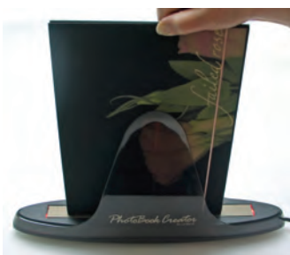
Figure 14: Krause holds the cover in the thermal binder to melt the glue and adhere the pages to the spine.
