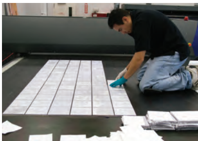
Figure 26: Placing tiles on UV-flatbed printer at Colorado Plastics.
